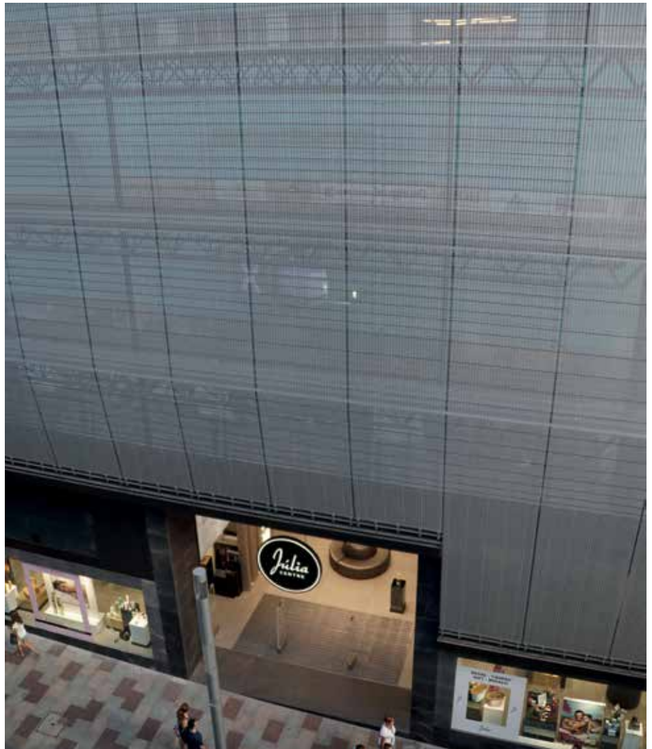
W.S. Tyler Architectural Mesh allows extensive façades to be clad with a homogenous appearance.
