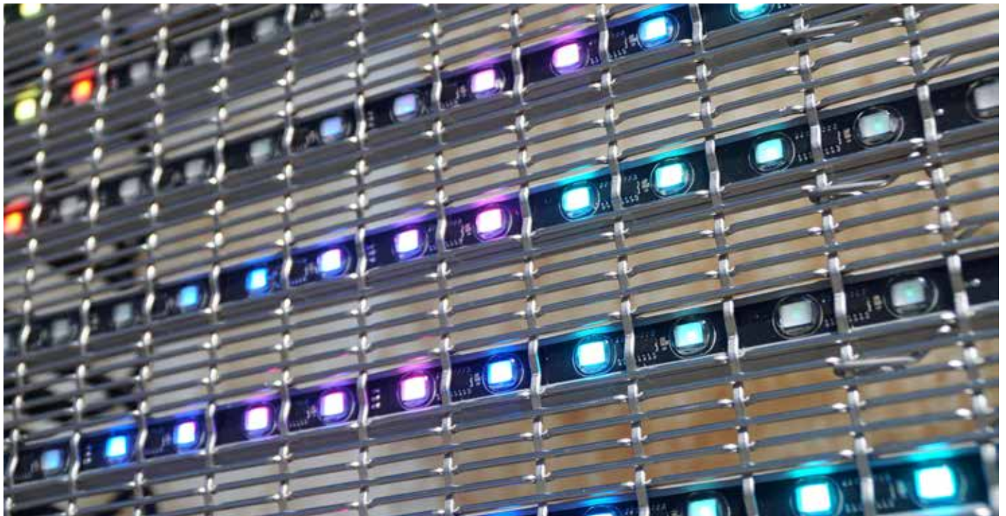
Close-Up: IMAGIC WEAVE® LED technology.
